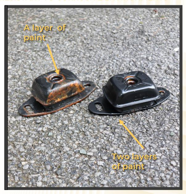
Anticorrosive treatment equivalent to stainless steel: The metallic parts are also treated with Anticorrosive treatment of Zinc Nickel according to DIN 50962-Fe // Zn-Ni (12) // A (800h Salt Fog Chamber). On which 2 layers of PU (Polyurethane) paint are added to ensure protection equivalent to Aisi 304 stainless steel.
